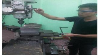
5. Drilling of metal plates and blocks using milling machine
