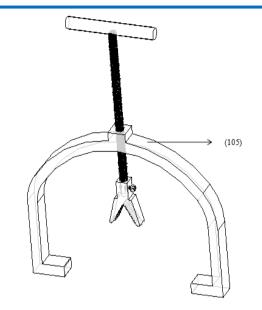
Figure 6. Schematic view of the structure of the U-Frame
