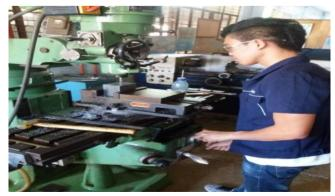
4. Squaring of metal plates and metal blocks using milling machine
