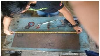
2. Laying out of the design and sizes directly to materials using scriber and steel rule
