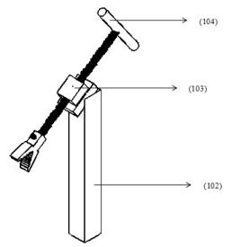
Figure 4. Schematic view of the Structure of the Clamping support Assembly and Clamping Support Guide
