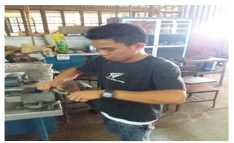
6. Threading of holes and shafting using tapping and die tools
