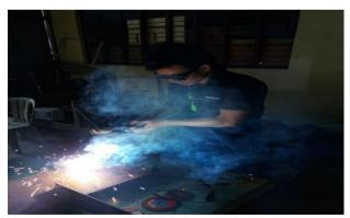
8. Welding the sub-assembly of clamp support guide using arc welding machine
