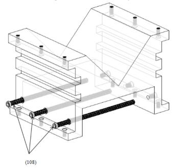
**Figure 9. Schematic View of the Structure of the Clamping Bolts**
