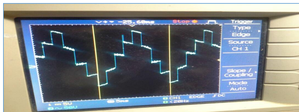
Figure 20. The Output Voltage Waveform of the Implemented Cascaded H-Bridge Inverter
