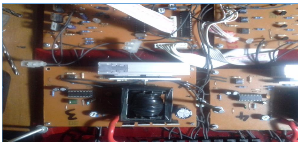
Figure 5. The Implemented Circuit of the Five Level Cascaded H-Bridge Inverter
