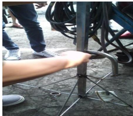
**5. Clean the welded portion of the boom and the sensor holder. This is to done to ensure a tight and mounting angle for a better stand of the device**
