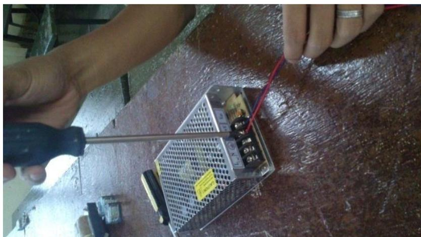
**8. Install the power supply going to the sensor, PLC, relay and siren. Ensure that the connections are tight and correct according to the polarity**
