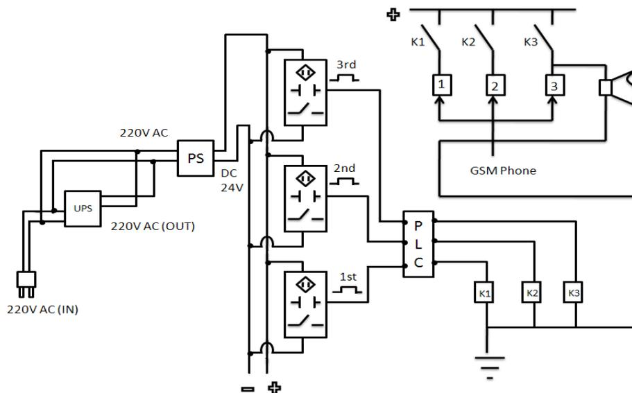
**Figure 3. Schematic Diagram of the Water Level Sensing and Warning Device with Short Message Service (SMS) Notification**
